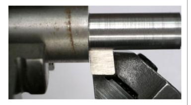
Never grind the tool bit too short. Always ensure the tool bit is long enough to protrude through the bottom of the holder. The clamp can be severely damaged if there is a jam up and the tool bit has been ground too short.
