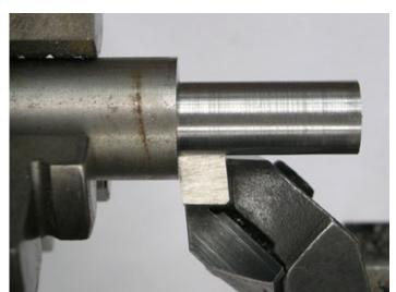
In the case of a severe jam, the tool bit will normally be forced down into the holder, avoiding serious damage to the workpiece and tool. In normal circumstances, the tool bit will not slip, even under heavy or intermittent cutting.
