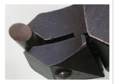
A cheap source of round HSS is broken or blunt center drills – No. 3 drills are  $\frac{1}{4}$  in diameter.
