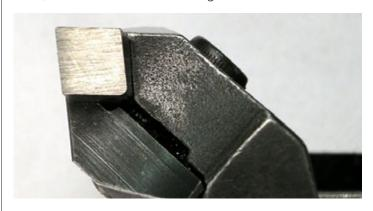
The tool bit can be ground on both ends. A radius point could be ground on one end and a sharp corner on the other. Just turn the bit over for a different profile.
